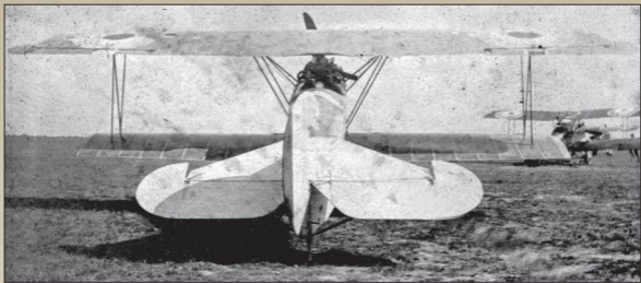
Rear view of Albatros built Fokker D.VII 817/18 'Neckchen IV' after being repainted in RAF markings. The bottom wing appears to have blue rib tapes while the top wing appears to have rib tapes cut from lozenge material.
