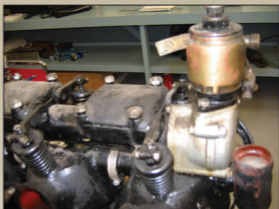
Large air pump (E29) characteristic of the 180hp Daimler Mercedes D.IIIa.
