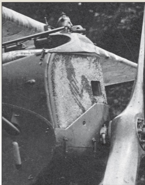
Radiator detail from the late production Fokker D.VII (Alb) shown on page 22.
