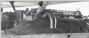
Cockpit coaming and LMG 08/15 'Spandau' detail from the Fokker D.VII (Alb) seen on page 9. Note the protective padding and twin filler caps.
