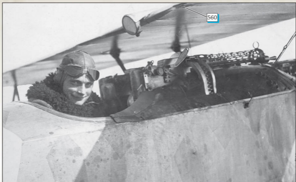
A smiling pilot, previously identified as Wilhelm Reinhard although this is now far from certain, sits in his Albatros built D.VII. Note the rear view mirror (E40), twin aileron control cables, LMG 08/15 'Spandau' details and 'washed out' appearance of the 4 colour fuselage lozenge fabric most likely indicating a tinted glaze coat (E). An Albatros style ZAK inspection window (560) can be seen under the trailing edge of the top wing.
