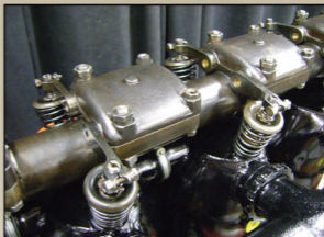
Overhead camshaft and valve gear rocker details.
