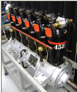
Water jacketed intake manifold and carburetor detail. A mount for the generator (P43) can be seen at right but the actual generator was very rarely installed in fighter aircraft unless used to power an electrically heated flight suit or wireless transmitter.
