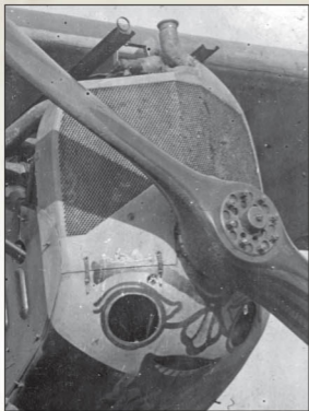
Radiator detail from D.VII. Note the holes cut into the chin cowl for additional cooling.
