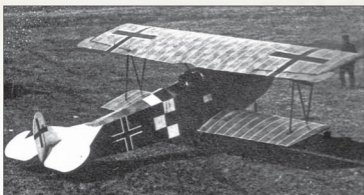
This unidentified late production Albatros built Fokker D.VII is believed to be from Jasta 43. Note the rigging guide doped to the right side of the fuselage (a trait associated with some Albatros built D.VII), top wing balkenkreuz location and pale (blue) rib tapes. All following archive photos are of Daimler-Mercedes powered Albatros built aircraft (unless noted otherwise).
